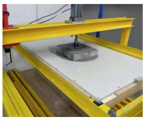
Tests have shown that the Impey Aqua-Dec EasyFit will easily support over 300kg (47 stone) without the need for under boarding
